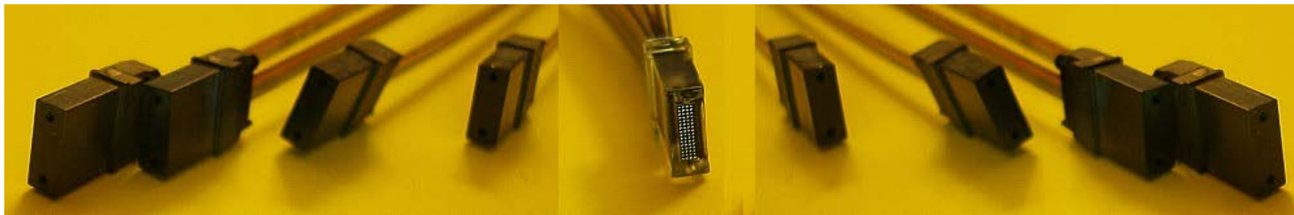
A 64 fiber ferrule fans out to 8 separate cables each with 8 fibers (4Tx and 4Rx)
